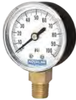
Dry Pressure Gauge 2" Dial & 1/4" Lower Mount
